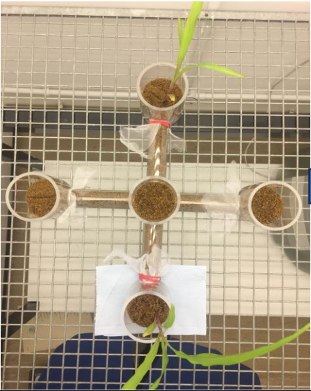
Soil olfactometer bioassay
