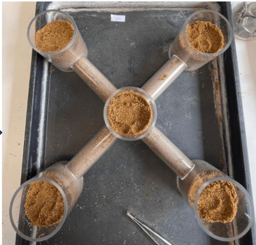
Soil olfactometer bioassay (Blend of odours in the form of chemicals, instead of plants)
